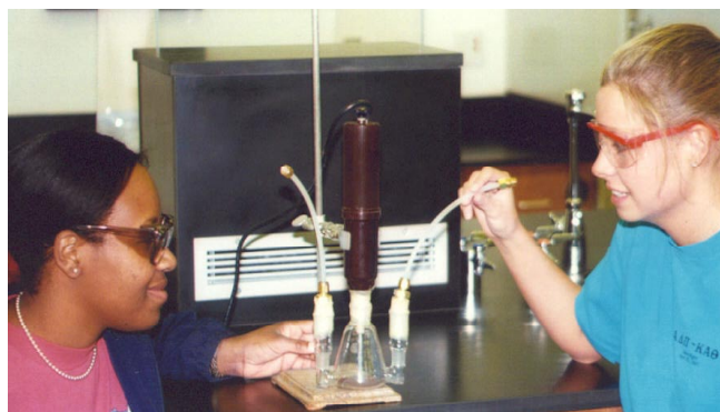
Figure 1. Two students look at the experimental setup that contained a high voltage discharge and a reaction vessel that produced nanotubes. They were told that their small start-up company had designed, built, and demonstrated the device for nanostructure synthesis. In undergraduate research projects, students have used this simple system to produce nanostructures from metal/hydrocarbon mixtures, ozone from oxygen/nitrogen/argon mixtures and amino acids from ammonia/methane/water mixes.
